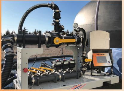
QuickDraw Max is a fully automated sprayer tender system. Start by creating a recipe - that is the applied application rates/hectare for each chemical in the batch. Recipes are saved and used every time you load that mix of chemicals. Enter the application rate/hectare you will be spraying and the size of load you need, either in total litres or total hectares to spray. QuickDraw
